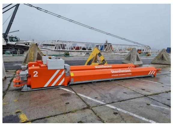
Source: Supplied | Four Hydraulic Shore Tension Units currently in use at the Port of Cape Town
