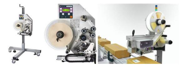
Print and apply labellers eliminate the need for employees to print and stick labels onto products and packaging. Instead, labels carrying barcodes, serial numbers, QR codes, personalised messages and even graphics are applied directly to packaging. This means manufacturers can print and apply labels on-demand, reducing storage needs for stock and product variant labels.
