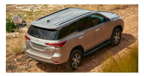
Another marked improvement is the use of a knob on the facia to select low range instead of the outdated short gear lever of the previous model. Ground clearance is 225mm and approach and departure angles are 29 and 25 degrees. One of the biggest criticisms of the previous Fortuner was the fact that it was so closely related to its work-horse Hilux brother, both in appearance and ride. The new Fortuner spins all that away into history.
