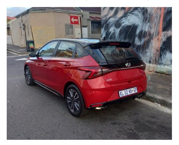
The i20 N Line is a turbocharged three-cylinder front-wheel drive that gives an output of 90kW and 172Nm. It's linked to a seven-speed dual-clutch transmission (DCT), which can be used in manual shift with paddles on the steering.
