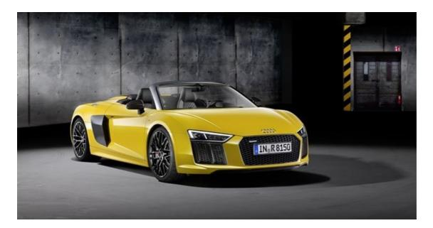
The R8 Spyder weighs in at only 1720kg, thanks to its ultra-light multimaterial Audi Space Frame, which has been constructed with a combination of aluminium and carbon fibre reinforced polymer (CFRP). The soft top itself is an anorexic 44 kilos, and is capable of opening and closing in 20 seconds, at speeds of up to 50km/h.
