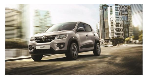
There are two models to choose from, Expression and Dynamique, both powered by the same 1.0-litre, 3-cylinder engine, that churns out 50kW at 5,500 rpm and 91Nm at 4 250rpm and is linked to a five-speed manual gearbox.
