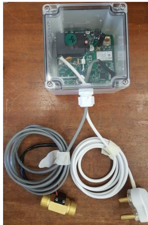
A smart meter that measures and reports water use by the minute. Author supplied
