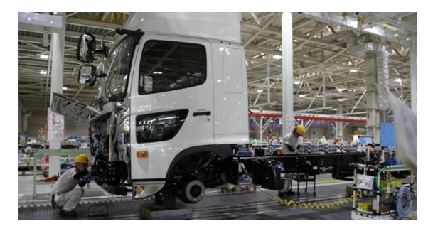
This is a world-class, state-of-the-art truck manufacturing facility with a high proportion of robotisation – including 95% of the cab welding and 95% of the painting – to ensure the highest quality standards and production consistency. It includes more in-house manufacturing than previously to streamline and simplify assembly operations.
